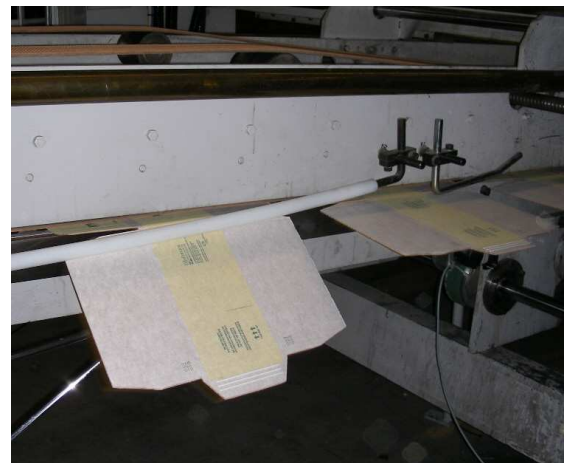
Example of a low pressure gluing system installed on a flexo folder- gluer machine
